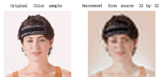
Fig.11 Left : sample 2, Right : recovered from 32x32 source density pixels, 0.92 correlation coefficient
