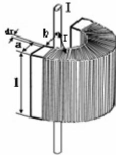
Fig.4 Constants of Current Viewer for Sensor Output Calculation
