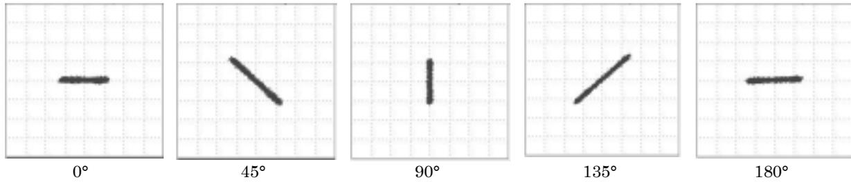
Fig.8 Lissajous Diagrams at each of Vector Current Viewer Angles (10kHz, 5A)
