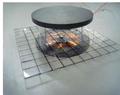
Fig. 4 Tested transformer employing the dish like ferrite cores.
