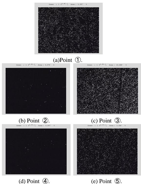
Fig.11 Extracted 1/f frequency fluctuations from the permalloy45%.
